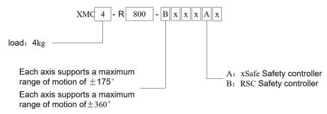
Figure 4-1. The model description of xMate SR4-C
