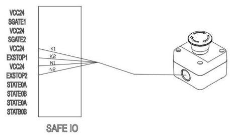
Figure 6-13 Emergency stop switch wiring diagram
