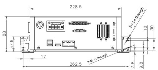
Figure 5-7 Horizontal installation
