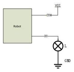
Figure 6-10 PNP output wiring diagram
