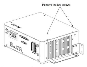
Figure 5-10 Removing screws
