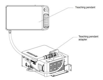
Figure 5-13 Schematic diagram of teaching pendant connection
