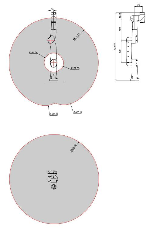
Figure 4-2 Working space of xMate SR4-C
