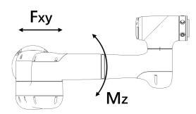
Fig 5-5 Supporting reaction force of the robot
