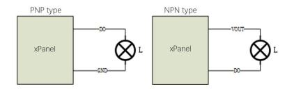
Figure 6-19 End effector output interface
