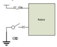
Figure 6-8 NPN input wiring diagram
