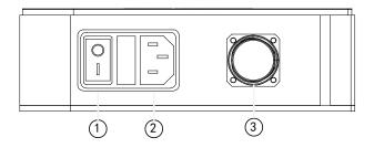
Figure 6-21 Power adapter interfaces
