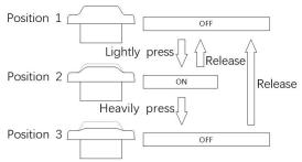
Figure 2-2. Positions of the enabling switch
