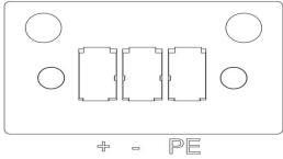
Figure 6-3 Power supply interface (side view for cables)
