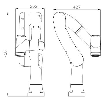
Figure 5-3 Reference transportation dimensions of the robot
