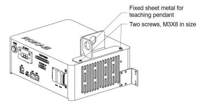
Figure 5-11 Installation of teaching pendant fixing sheet metal
