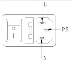
Figure 6-22 Power input interface
