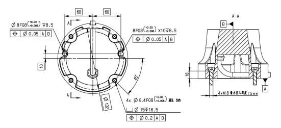
Figure 5-4 Reference bracket fixing method
