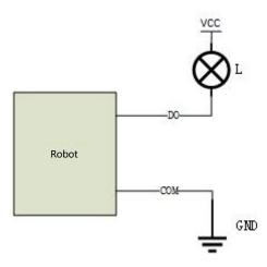
Figure 6-9 NPN output wiring diagram
