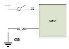
Figure 6-7 PNP input wiring diagram
