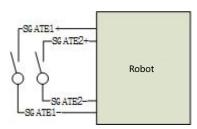
Figure 6-11 External emergency stop interface
