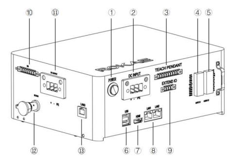
Figure 6-2 Controller interfaces
