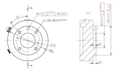
Figure 5-6 Tool flange installation
