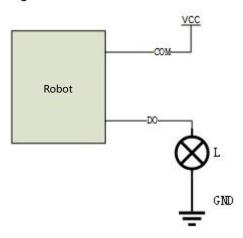
Figure 22. PNP output wiring diagram
