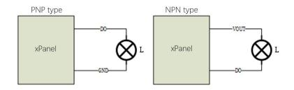
Figure 27. End effector output interface
