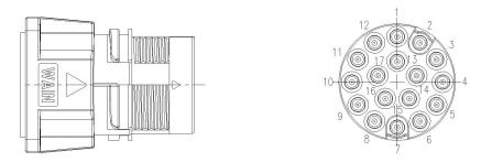
Figure 15. Handheld emergency stop and enabling device interface
