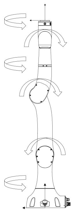
Figure 4. Definitions of robot rotation directions and coordinate systems for details). The definitions of axis rotation directions and coordinate systems are described below. Base coordinate system: The -X axis points in the outgoing cable direction of the base, and the +Z axis in a direction perpendicular to the mounting surface. The Y axis is determined by the right-hand rule.
