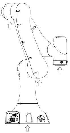
Figure 8. Robot pose and suggested points of force application during
