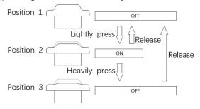
Figure 2-2. Positions of the enabling switch
