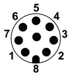
Figure 26. The end effector round connector interface
