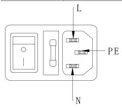
Figure 30. Power input interface
