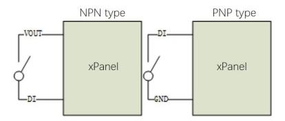
Figure 28. End effector input interface
