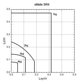
Figure 4-3. Maximum wrist payload and center-of-gravity shift
