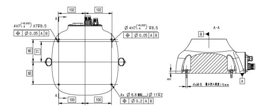
Figure 10. Reference bracket fixing method
