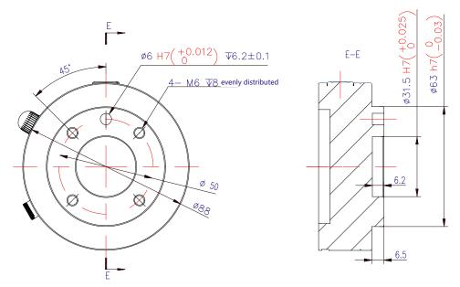
Figure 11. Tool flange installation
