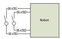
Figure 23. External emergency stop interface
