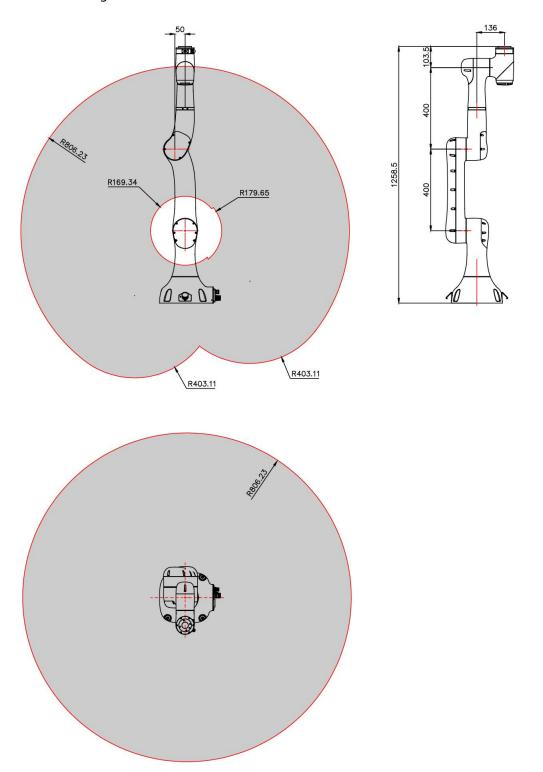
Figure 4-2. The working space of xMate SR4
