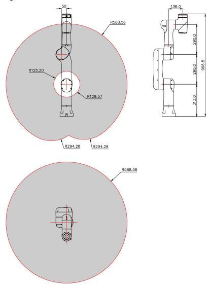
Figure 4-2 Working space of xMate SR3-C
