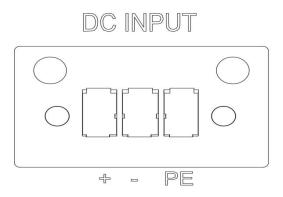
Figure 6-3 Power supply interface (side view for cables)
