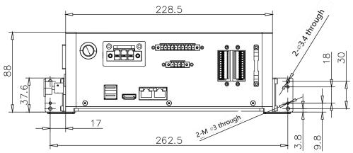
Figure 5-7 Horizontal installation
