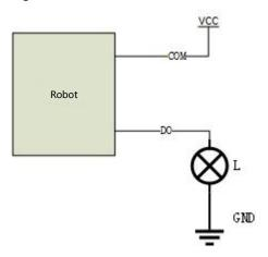
Figure 6-10 PNP output wiring diagram
