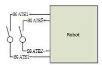
Figure 6-11 External emergency stop interface
