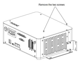
Figure 5-10 Removing screws
