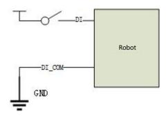
Figure 6-7 PNP input wiring diagram
