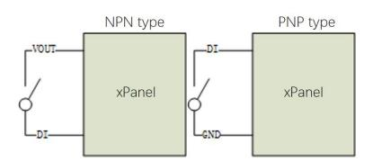
Figure 6-20 End effector input interface
