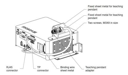
Figure 5-12 Installing the teaching pendant adapter harness
