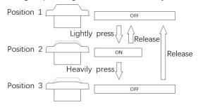
Figure 2-2. Positions of the enabling switch
