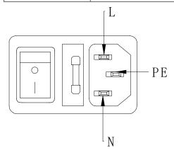
Figure 6-22 Power input interface
