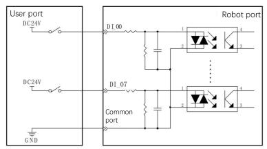
When the common port is 24 VDC, the NPN input signals are available, as shown below:
