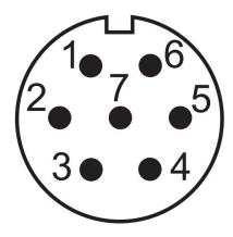
Figure 6-16 EtherCAT servo drive debug interface
