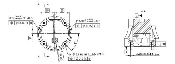
Figure 5-4 Reference bracket fixing method
