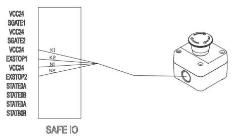
Figure 6-13 Emergency stop switch wiring
