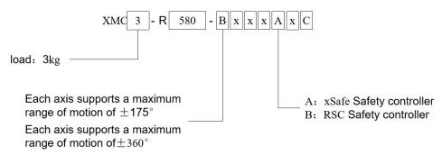
Figure 4-1. The model description of xMate SR3-C
