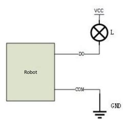
Figure 6-9 NPN output wiring diagram
