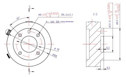
Figure 5-6 Tool flange installation
