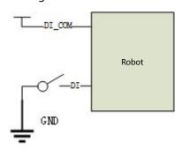
Figure 6-8 NPN input wiring diagram
