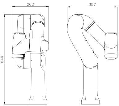
Figure 5-3 Reference transportation dimensions of the robot
