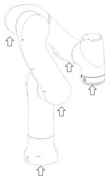
Figure 5-2 Robot pose and suggested points of force application during
