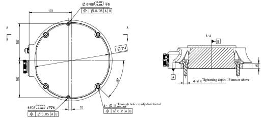
Put pins in the reserved cylindrical pin holes for accurate positioning. Then use four M10×35 hexagon socket head cap screws (strength grade 12.9) to fix the robot's base on the bracket.
