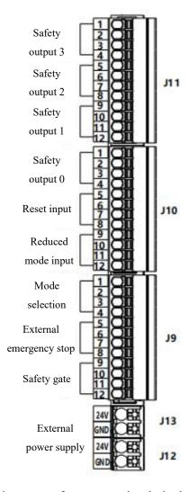
Each group of safety input or safety output signals is dual-channel redundant, so each group contains two inputs/outputs, namely "Loop 1" and "Loop 2", with a total of 4 terminals. Definition of pins:
