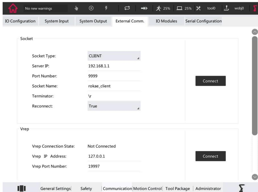
Fig. 20 External communication interface
