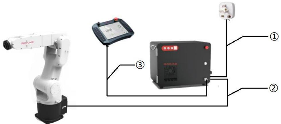
Fig. 22 Robot system cable connection
