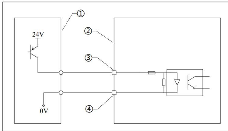
**Fig. 29 DI/DO high-level input wiring diagram**
