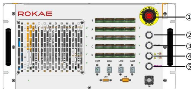
Fig. 34 XBC5M control cabinet buttons and indicators
