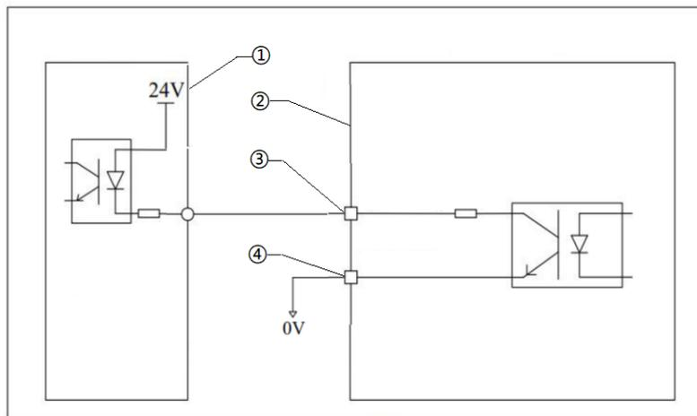
Fig. 32 DI/DO low-level output wiring diagram
