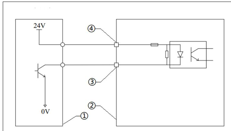
**Fig. 30 DI/DO low-level input wiring diagram**
