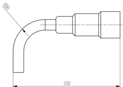
Fig. 15 The bending radius of the Teach Pendant cable
