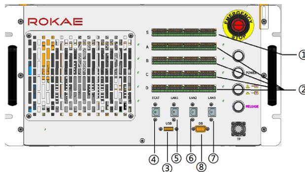
Fig. 17 Interfaces of the XBC5M control cabinet
