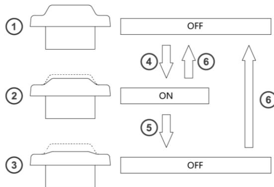
Fig. 1 Schematic diagram of the enabling switch
