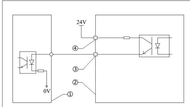
Fig. 31 DI/DO high-level output wiring diagram
