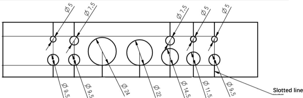
Fig. 25 XBC5 control cabinet - size of cable outlets
