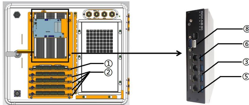
Fig. 16 Interfaces of the XBC5 control cabinet
