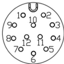
Fig. 40 Definition of LAN port pins
