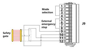
Users can connect safety door devices (photoelectric switches/limit switch/safety light curtains, etc.) through this interface. For example, when using a safety light curtain, as the interface is an active interface, simply connect the switch input and output circuit to the safety door interface.
