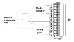
Users can connect emergency stop buttons or emergency stop handles through this interface. For example, when using the emergency stop button, as the interface is an active interface, simply connect the input and output circuits of the emergency stop switch to the external emergency stop interface, as shown in the above figure.
