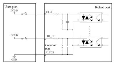
When the common port is 24 VDC, the NPN input signals are available, as shown below:
