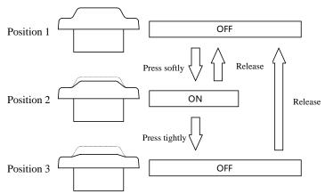
The enabling switch is located on the back of the Teach Pendant, as shown in 3.3.2.
