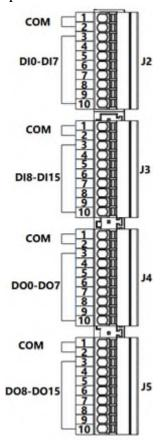
The control cab is equipped with 16 general-purpose digital inputs and 16 general-purpose digital outputs as standard, with pin definition as follows:
