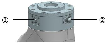
The Direct Teach mode can be enabled by pressing and holding the direct teach button.
