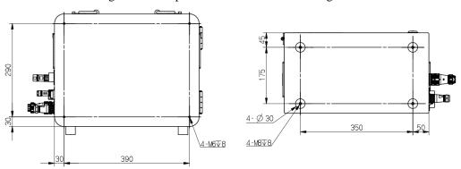
There are four M6 threaded holes in 8 mm depth on the back of the control cab and four M8 threaded holes in M8 depth at the bottom. The fixing mode shall be chosen according to the operating environment.
