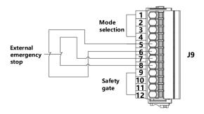
Users can connect emergency stop buttons or emergency stop handles through this interface. For example, when using the emergency stop button, as the interface is an active interface, simply connect the input and output circuits of the emergency stop switch to the external emergency stop interface, as shown in the above figure.
