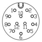
Fig. 36 Definition of PS1 pins
