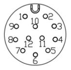
Fig. 34 Definition of LAN port pins
